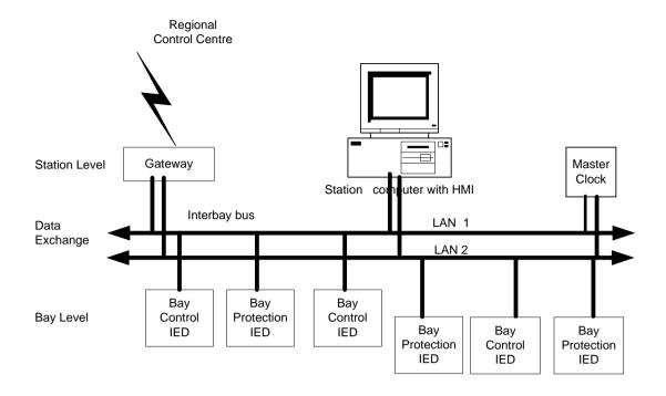
**System Architecture of Substation Automation**
